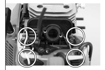
13.2 Remove pulse tube and protective spring from cylinder base.
